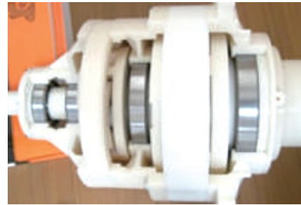
A working model of a modular planetary gear.
